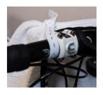
Attach the elastic around the handlebars or stem or head tube (around the handlebars in the picture).
